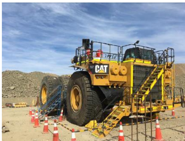
Candelaria new CAT 793F haul truck assembly
