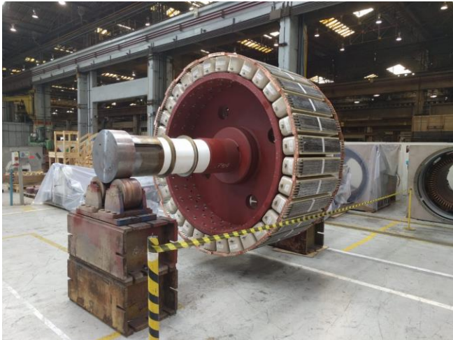
Ball mill motor replacements arriving on site
